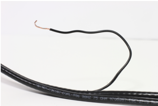
Figure 5: Messenger wire separated
